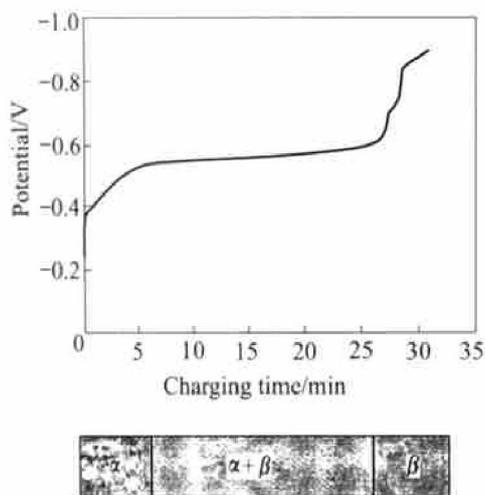
**Fig. 3** Dependence of electrode potential on charging time of Pt/MI/I/O films (Pt layer 20 nm, MI layer 945 nm, specimen size 0.8 cm × 0.6 cm; charging current density 1.25 mA/cm<sup>2</sup>, temperature 15 °C.  $\alpha$  phase corresponds to soluble hydrogen in MI bulk, and  $\beta$  phase to La dehydride and trihydride)
