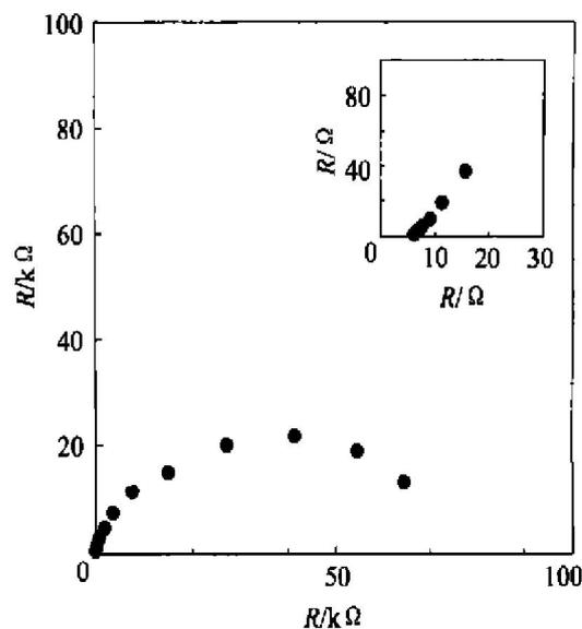
**Fig. 5** Electrochemical impedance spectrum of Pt/MI/I/O film (surface area of film electrode: 0.5 cm<sup>2</sup>)
