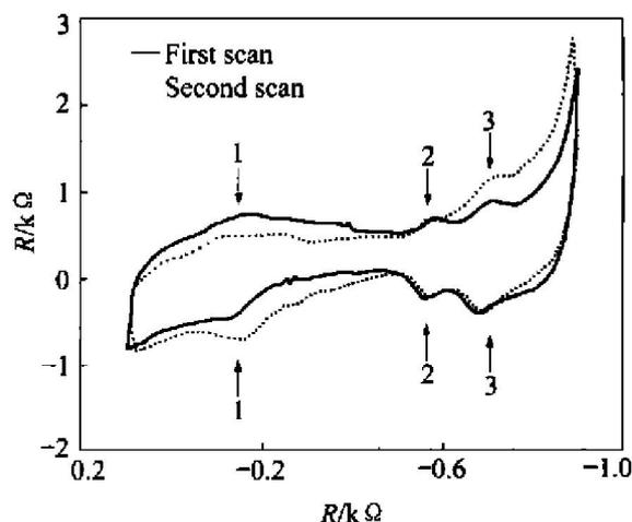
**Fig. 4** Cyclic voltammograph curve of Pt/MI/I/O film (Pt layer 20 nm, MI layer 945 nm, scan rate 100 mV/s, temperature 15 °C)
