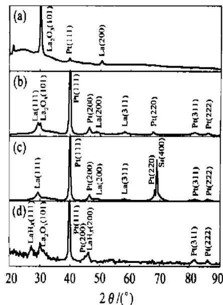
**Fig. 1** XRD patterns of different Pt/Ml films deposited on ITO and silicon slice substrate
