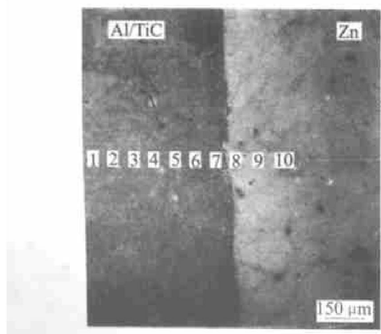
Fig. 3 SEM image for interface of prepared Al/TiC alloy and zinc alloy (Solidified from liquid maintained at 620 °C for 35 min)
