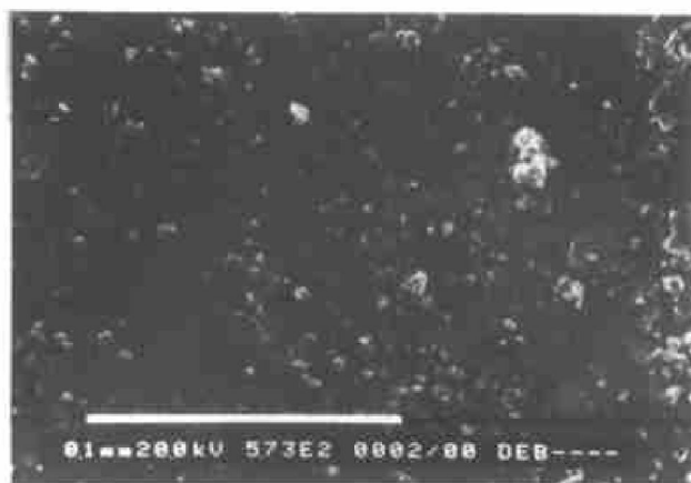
Fig. 3 Debris of TiAl based alloys nitrided at 940 °C for 50 h
