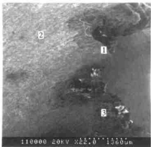
Fig. 4 SEM image of interface between enamels and aluminum alloy for sample S 2
