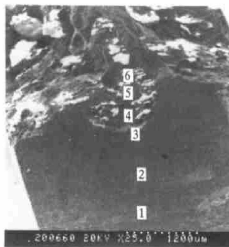
Fig. 6 SEM image of interface between enamels and aluminum alloy for sample S 3-1
