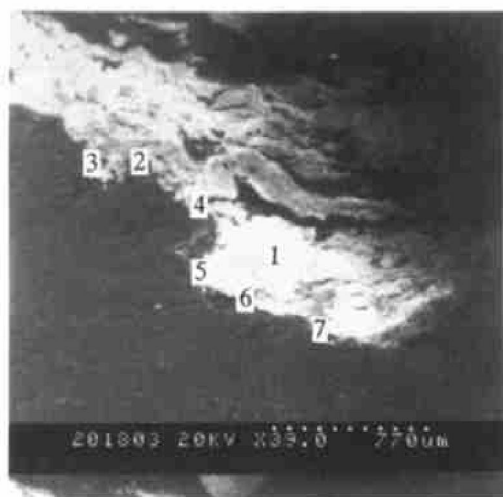
Fig. 7 SEM image of interface between enamels and aluminum alloy for sample S_4
