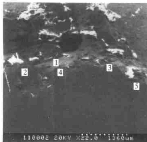
Fig. 5 SEM image of interface between enamels and aluminum alloy for sample S 3
