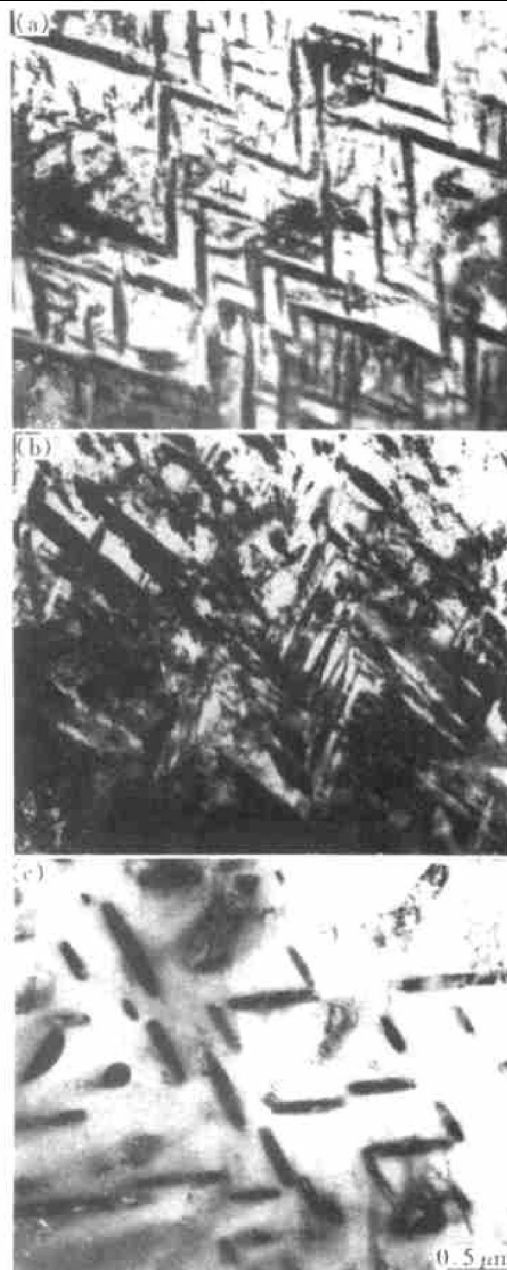
Fig. 3 Effect of ageing time on microstructure of Ti-15-3 alloy
