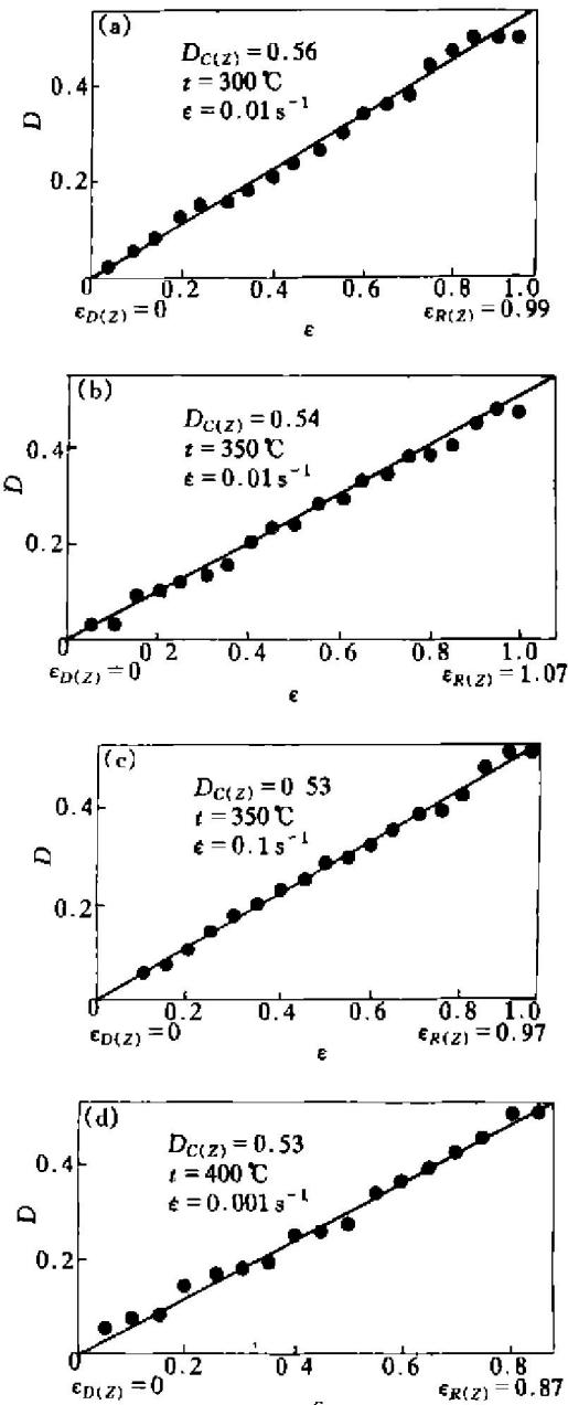
**Fig. 1** Comparison between model predictions and experimental results for damage evolution curves
