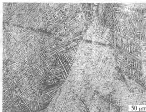
Fig. 4 Micrograph of weld metal by F-PAW
