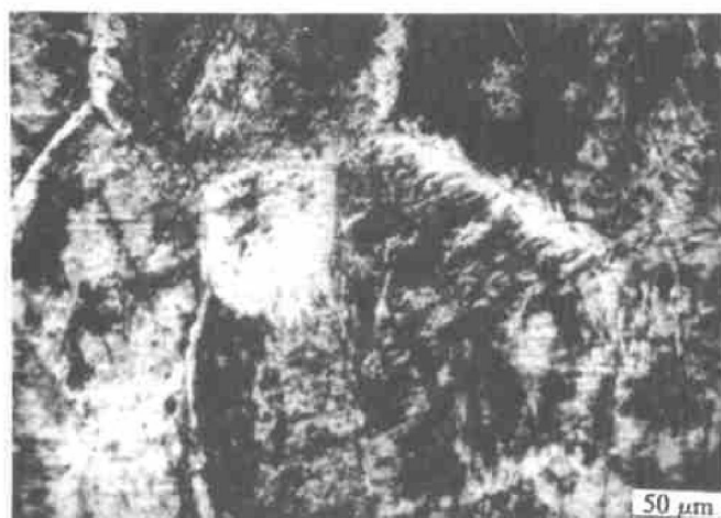
Fig. 2 Micrograph of weld metal by M-GTAW
