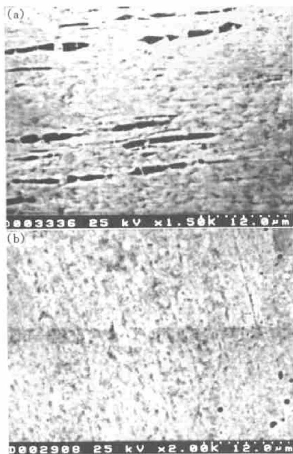
Fig. 3 Microstructures of commercial cathode and nanocomposite cathode
