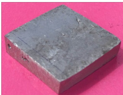
Fig. 6 Image of A380 die casted part
