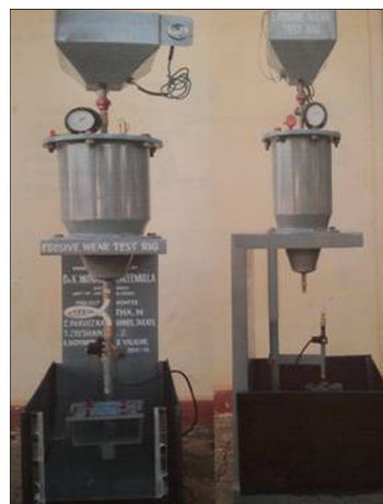
Fig. 1 Erosive wear test rig developed for erosion test
