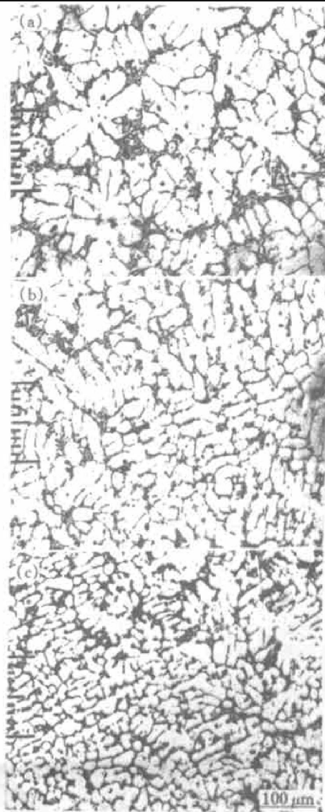
Fig. 4 Solidification structure of A356 alloy with MTT (LTM is stirred at different temperatures) (a) –600 °C; (b) –640 °C; (c) –680 °C
