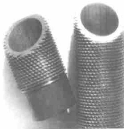
Fig. 1 3D outside fin copper tube machined by pre-roll ploughing
