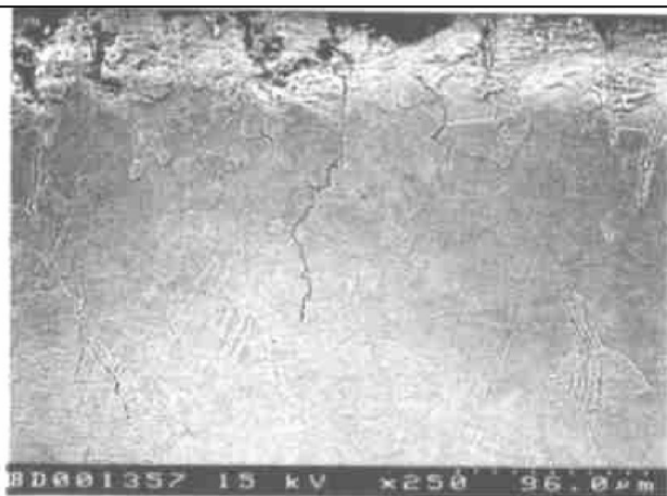
Fig. 2 Fatigue crack located on longitudinal section of pure titanium sample
