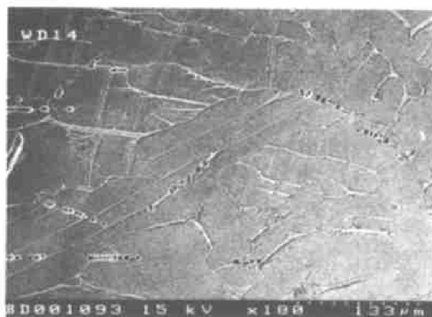
Fig. 4 Two-dimensional morphology of spherical voids after vacuum annealing
