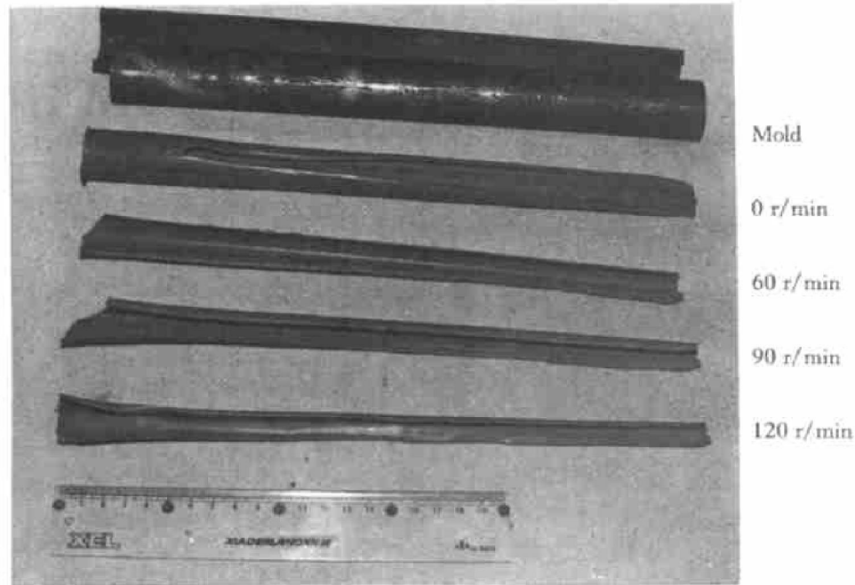
Fig. 6 Wax models formed under different rotating speeds
