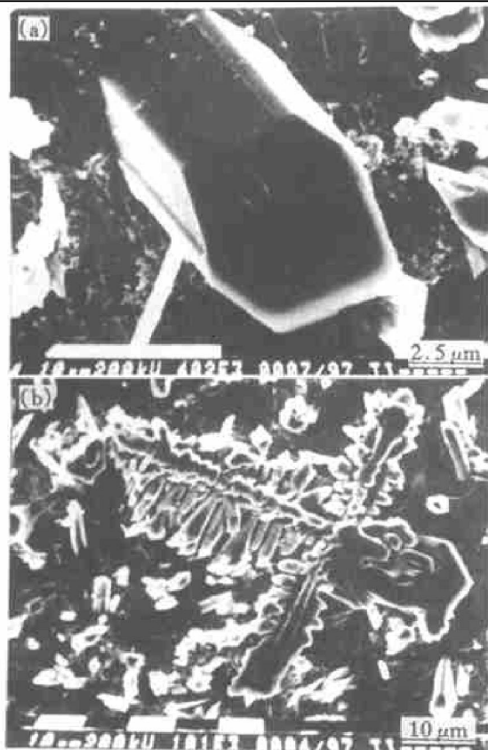
Fig. 2 Typical morphologies of TiB (a) and TiC (b) in TMCs
