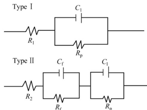
**Fig.5** Equivalent circuit diagrams for analysis of measured impedance with variation of surface condition ( $R_1$ : Total resistance of solution and mortar;  $R_p$ : Polarization resistance;  $C_1$ : Double-layer capacitance;  $R_2$ : Solution resistance;  $C_f$ : Film capacitance;  $B_f$ : Film resistance)
