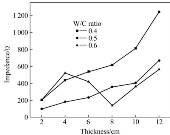
**Fig.4** Variation of impedance at 100 kHz as function of thickness and W/C ratio
