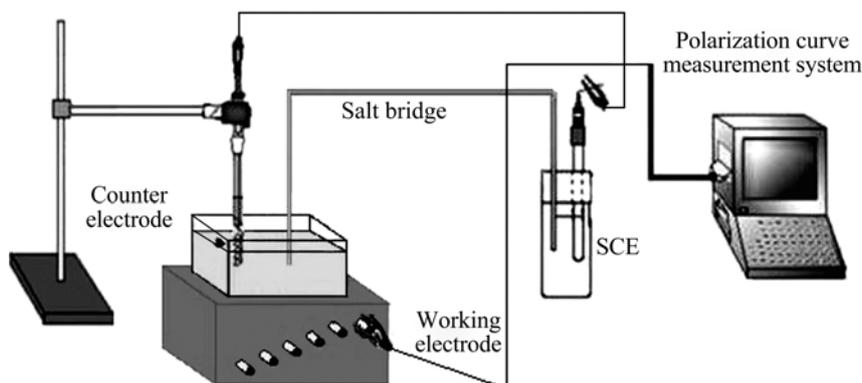
**Fig.1** Experimental apparatus for measuring corrosion potential and impedance
