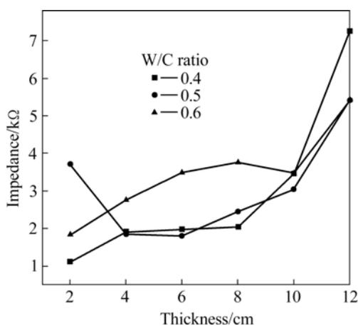
**Fig.6** Variation of impedance at 10 mHz as function of thickness and W/C
