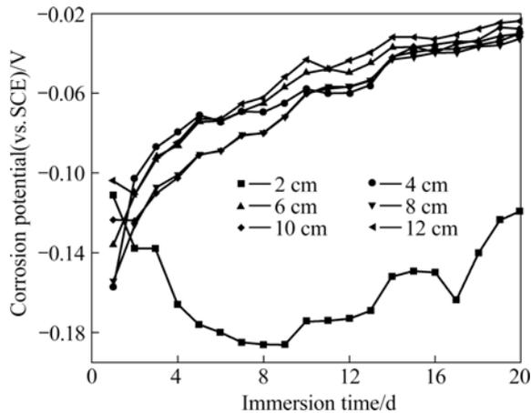
**Fig.2** Variation of corrosion potential as function of thickness with immersion time in natural sea water solution (W/C ratio: 0.4)
