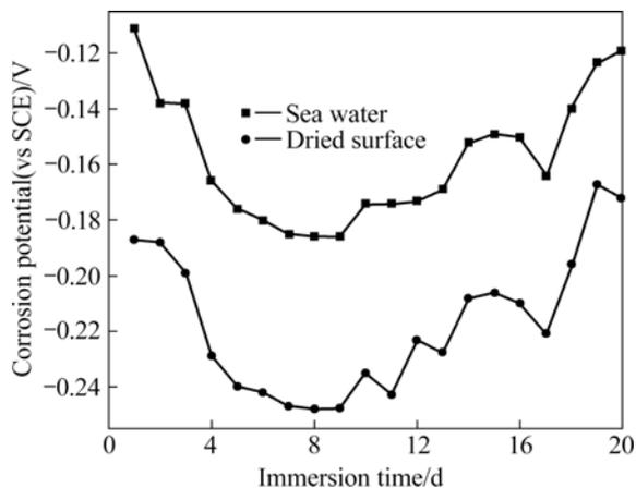
**Fig.3** Variation of corrosion potential measured with reference electrode immersed in sea water solution or placed on outer dried surface (Cover thickness: 2 cm; W/C ratio: 0.4)
