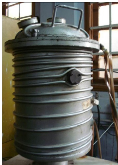
Fig. 2 Vacuum chamber surrounded by copper tubes for water circulation provision
