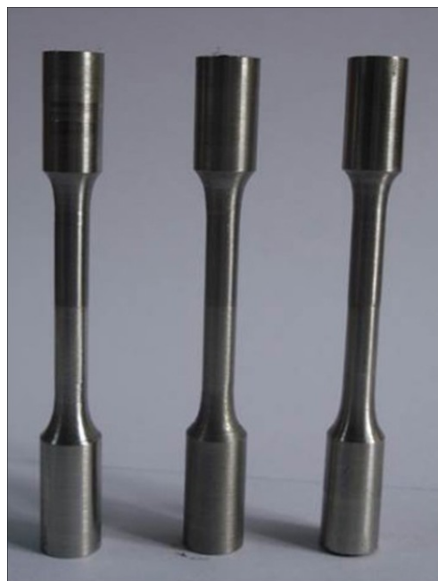
Fig. 5 Typical tensile specimens machined out of tensile sample of DSJs of TA and SS
