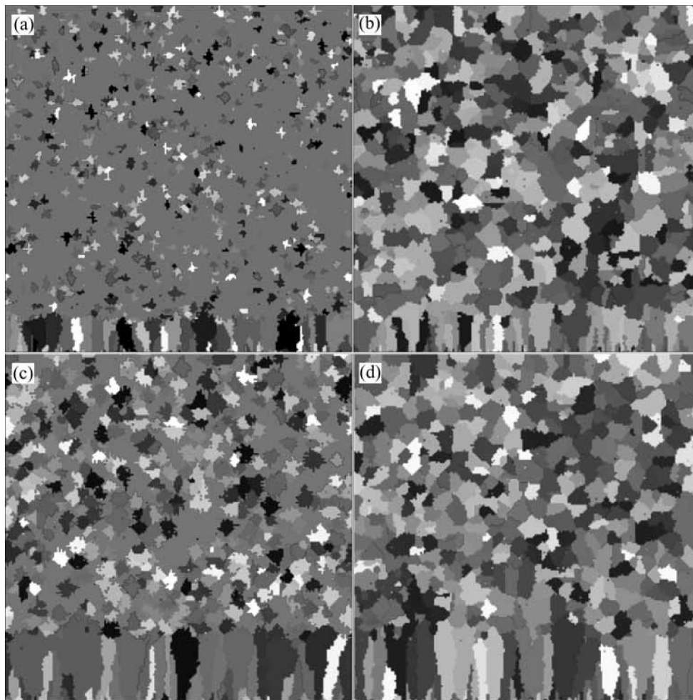
Fig.7 Microstructures with \theta_2=1\ 383\ ^\circ\text{C} and \theta_3=1\ 340\ ^\circ\text{C} respectively: (a) and (b) at \dot{\theta}=0.08\ ^\circ\text{C/s} ; (c) and (d) at \dot{\theta}=0.03\ ^\circ\text{C/s}
