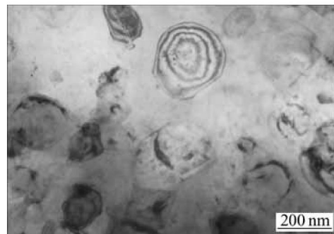
Fig.3 TEM image of melt-spun Cu75Cr25 ribbon (Velocity of cooling roller is 33 m/s)
