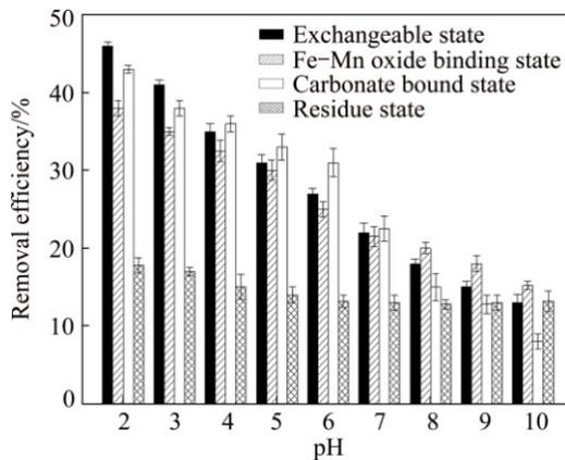
Fig. 5 Various forms of Pb removal at different pH values
