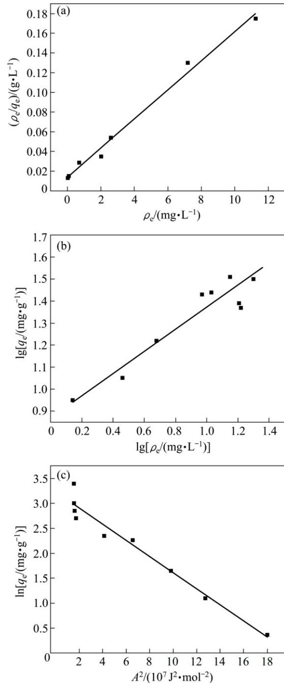
Fig. 6 Langmuir adsorption isotherm (a), Freundlich adsorption isotherm (b) and Dubinin–Raduskevich adsorption isotherm (c)
