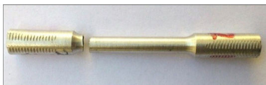
Fig. 21 Fracture mode of NC Al sample under tensile load
