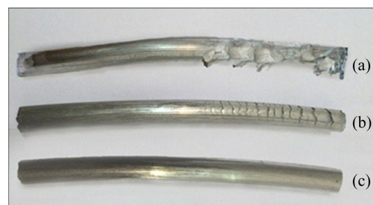
Fig. 3 Al5083/B 4 C nanocomposite extruded under different conditions: (a) 640 °C and extrusion rate of 1.5 mm/s; (b) 550 °C and extrusion rate of 3 mm/s; (c) 550 °C and extrusion rate of 1 mm/s
