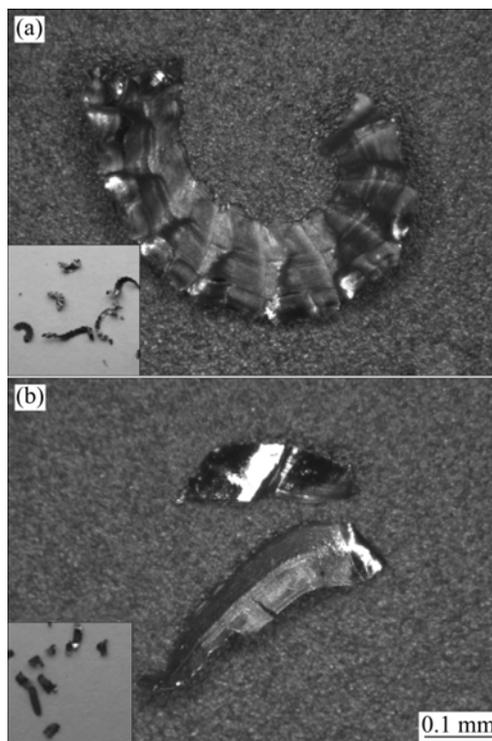
**Fig.7** Configuration of chips under high speed machining of Ti-6Al-4V: (a) Without nitrogen gas; (b) With nitrogen gas
