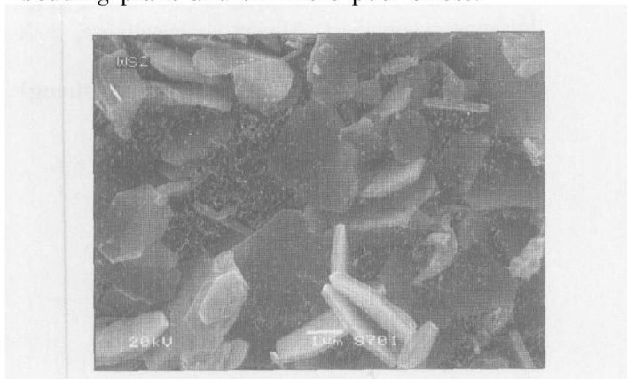
Fig. 8 Microstructure of WS 2 powder
