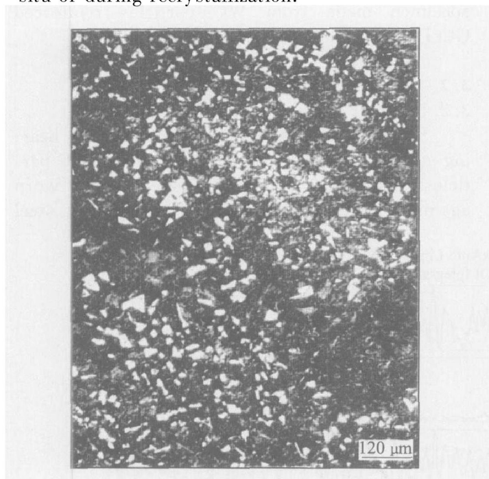
Fig. 1 Microstructure of WC/ steel matrix composite at lower magnification
