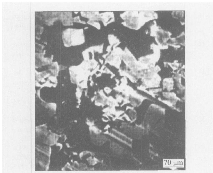
Fig. 11 SEM morphology of intragranular crack of coarse WC p on worn surface
