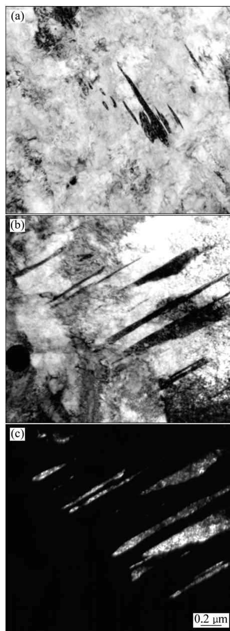
图 3 15-5PH 不锈钢在 550 °C 时效不同时间后的 TEM 像 Fig. 3 TEM images of 15-5PH stainless steel aged at 550 °C for various time: (a) Aging for 1 h; (b), (c) Bright field and dark field images showing the reversed austenite in martensite matrix aging for 8 h, respectively
