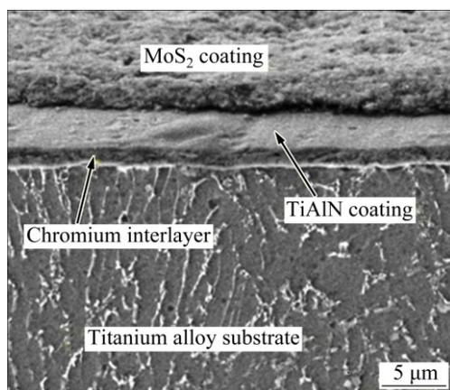
Fig. 6 SEM image on cross section of MoS<sub>2</sub>-coated surface along with TiAlN composite coating and chromium as interlayer
