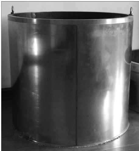
图 5 真空热胀形模具和转子屏蔽套照片 Fig. 5 Photo of die and rotor can during vacuum hot bulge forming
