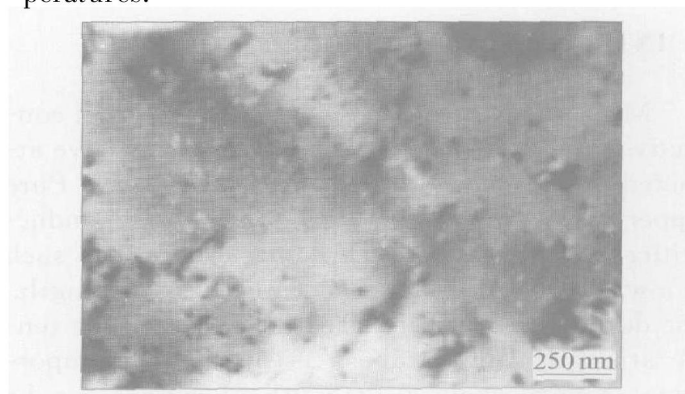
Fig. 1 Alumina particles in 0.12% ADSC (As-extruded)
