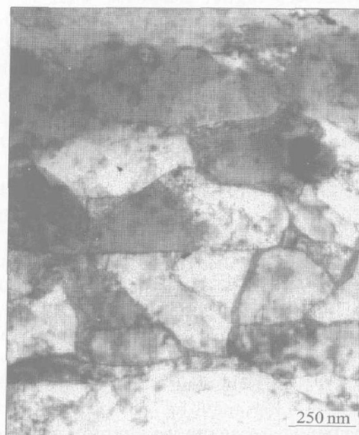
Fig. 6 Micrograph of 0.12% ADSC after annealing at temperature of 1000 °C
