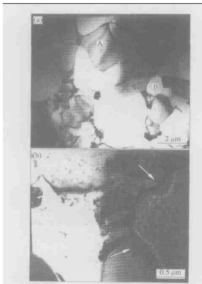
Fig. 9 TEM images of grains at elongation of 116.7%
