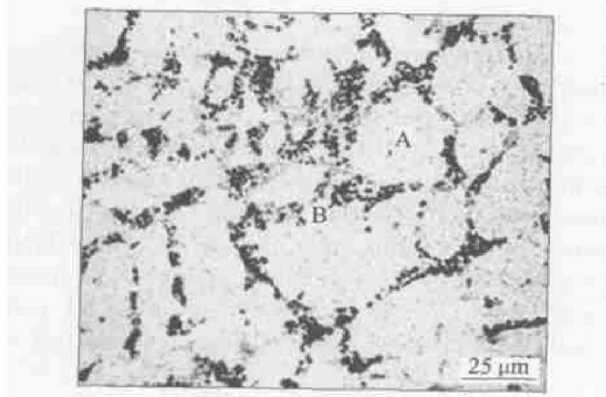
Fig. 1 Optical micrograph of as-cast Ni 50 Ti 45 Ta 5 SMA
