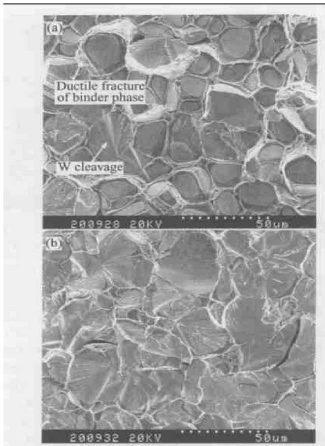
Fig. 10 Fractographs of tensile fracture surfaces for sintered samples after heat-treatment in vacuum (a) —Sample I; (b) —Sample II
