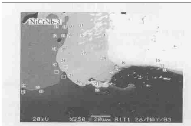
Fig. 5 Back-scattered electron image of \text{Ni-Cr-Nb} diffusion triple after annealing at 1 423 K for 170 h
