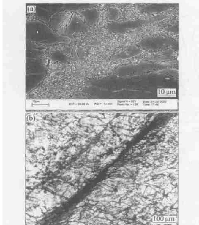
Fig. 3 Microstructures of shear bands at 185 °C and different strain (a) —Sample NR, 0.60; (b) —Crack in sample ZY, 0.80
