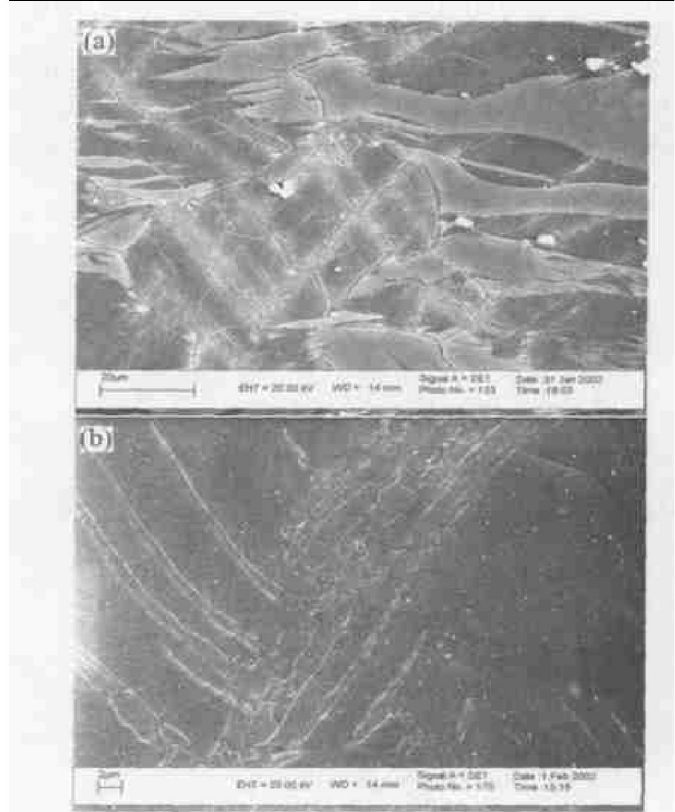
Fig. 7 Relationship of shear bands with \{10\bar{1}1\} twins at strain of 0.25 (a) —TR, 97 °C; (b) —ZY, 185 °C
