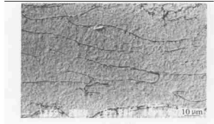
Fig. 5 Cross-sectional morphology of tungsten coating formed via induction plasma spraying of coarse powder
