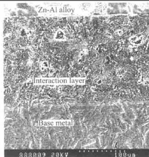
Fig. 5 Microstructure of interaction interface between Zn-Al alloy and \text{Al}_2\text{O}_3/\text{6061Al} composite
