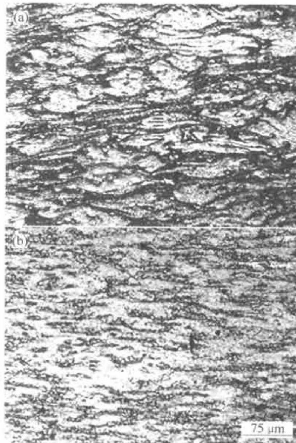
Fig. 4 Optical micrographs of Mg-alloy AZ91 compressed at different temperatures and constant strain rate of 0.05 \text{ s}^{-1} (a) —573 K; (b) —673 K
