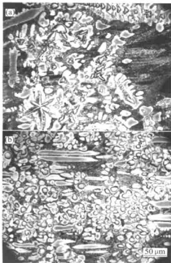
Fig. 7 SEM photographs of Cu-5.6% Cr (a) — R = 60 \mu\text{m/s} ; (b) — R = 200 \mu\text{m/s}
