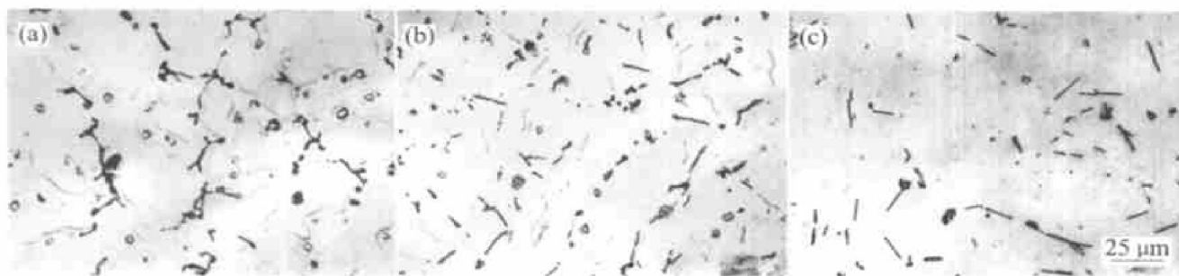
Fig. 1 Microstructures of as cast state (a) AZ61, (b) AZ61+ 0.7La and (c) AZ61+ 0.6Nd
