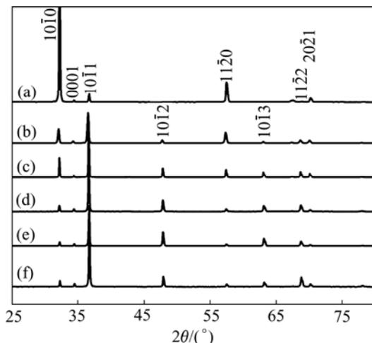
Fig.4 XRD patterns of AZ31 Mg alloy before and after ECAP: (a) Before ECAP; (b) One pass; (c) Three passes; (d) Five passes; (e) Seven passes; (f) Eight passes
