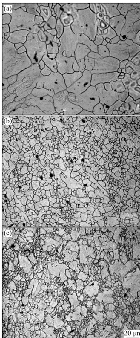
**Fig.1** Typical microstructures of ECAP AZ31 Mg alloys as function of die angle via route  $B_c$ : (a) Original unpressed morphology; (b) 4-pass through  $90^\circ$  die; (c) 4-pass through  $120^\circ$  die
