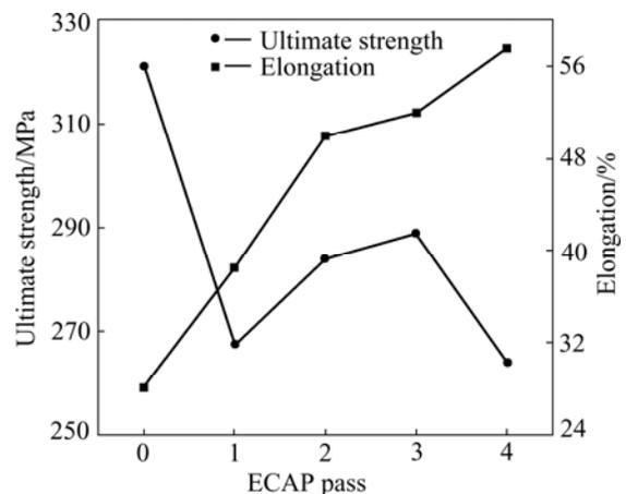
Fig.5 Mechanical properties of AZ31 Mg alloy as function of passes of ECAP
