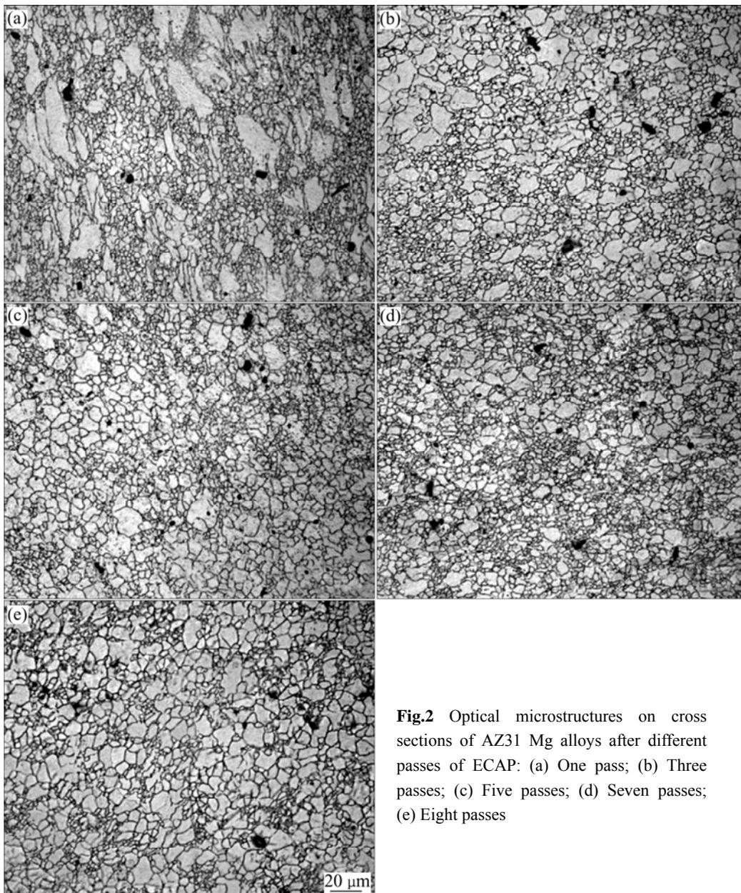
**Fig.2** Optical microstructures on cross sections of AZ31 Mg alloys after different passes of ECAP: (a) One pass; (b) Three passes; (c) Five passes; (d) Seven passes; (e) Eight passes
