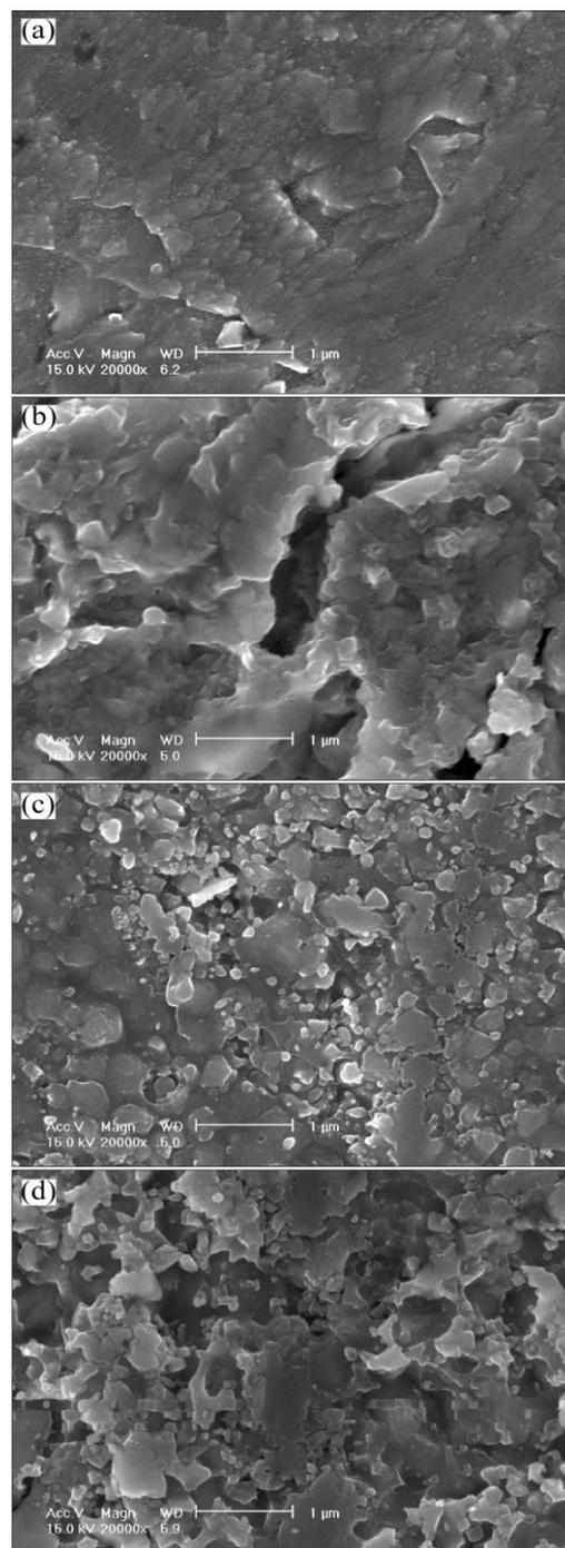
**Fig. 8** SEM images of Cu and Cu–CNT etched cross-section surface: (a) Cu; (b) Cu–1%CNT; (c) Cu–5%CNT; (d) Cu–10%CNT
