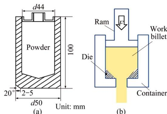
Fig. 2 Schematic diagram of extrusion process: (a) Billet shape; (b) Extrusion processing
