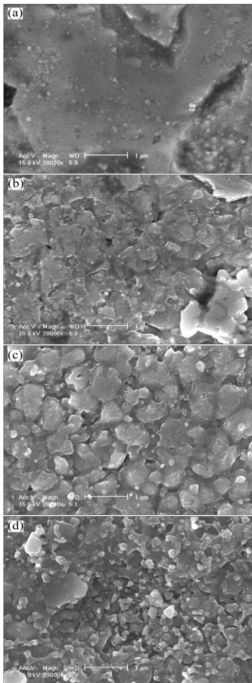
**Fig. 7** SEM images of Cu and Cu–CNT etched longitudinal section surface: (a) Cu; (b) Cu–1%CNT; (c) Cu–5%CNT; (d) Cu–10%CNT
