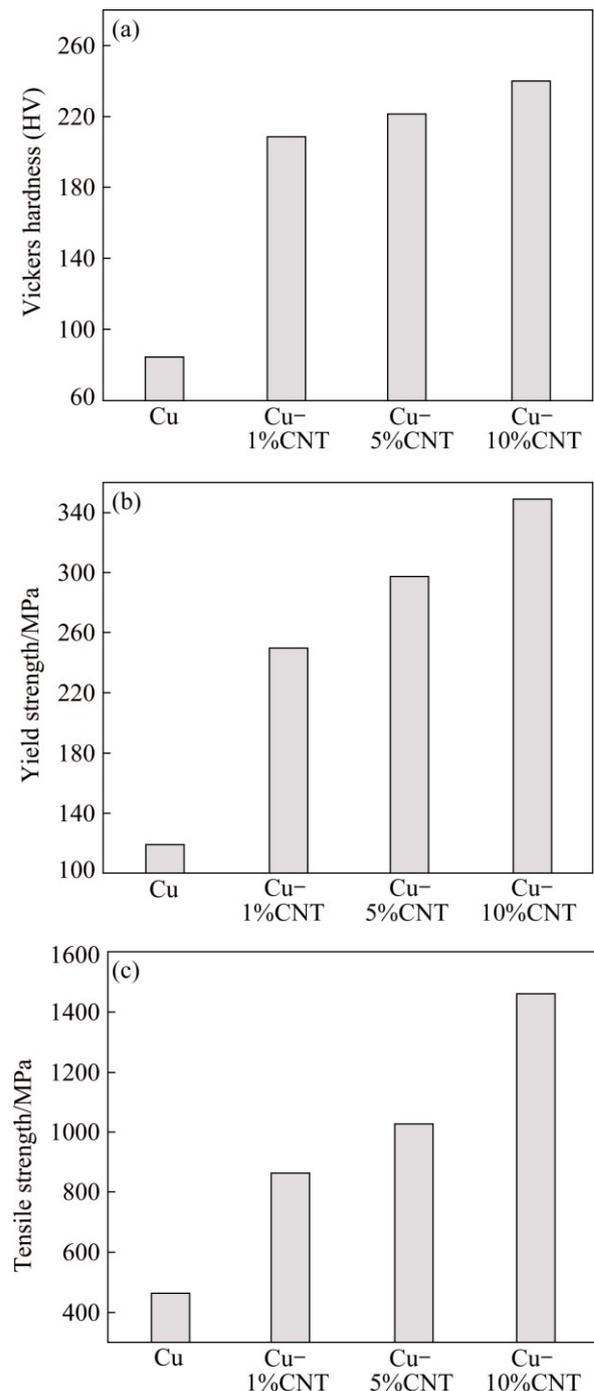
Fig. 10 Results of indentation test: (a) Hardness; (b) Yield strength; (c) Ultimate tensile strength
