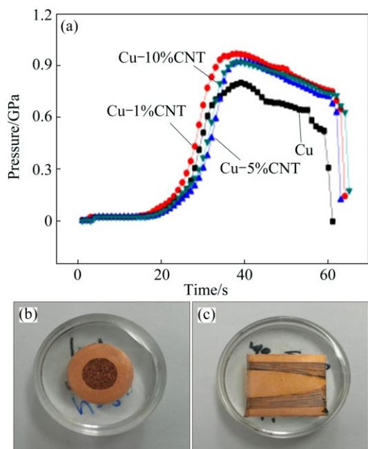
**Fig. 4** Results of extrusion test: (a) Extrusion curve; (b) Photograph of longitudinal section; (c) Photograph of cross-section
