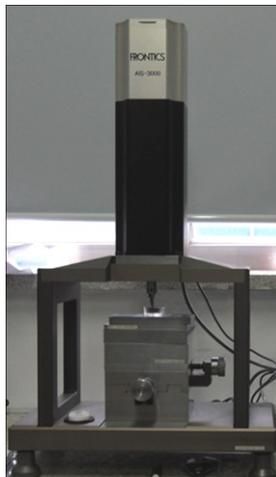
**Fig. 3** Indentation test equipment
