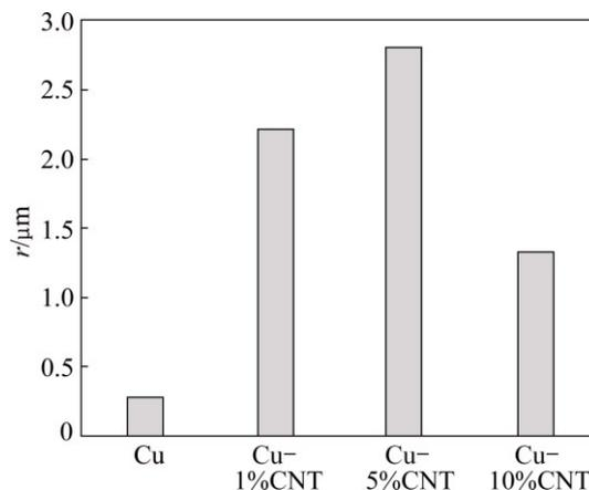
**Fig. 5** Size measurement graph of nano powders
