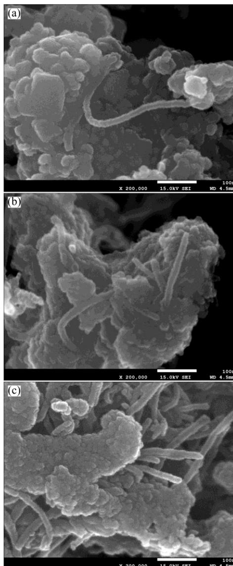
**Fig. 6** SEM images of Cu–1%CNT (a), Cu–5%CNT (b) and Cu–10%CNT (c) composites
