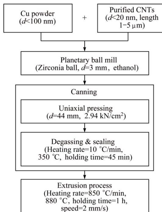
Fig. 1 Flow chart of fabrication procedures of CNT/Cu composites
