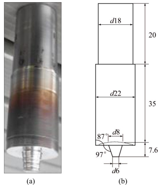
Fig. 1 Welding tool (a) and its geometry (b) (unit: mm)
