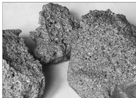
Fig.1 Photograph of coarse Al-Si alloy
