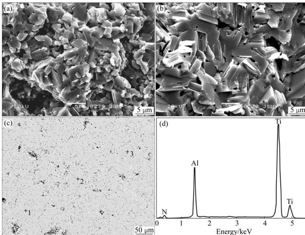
**Fig.3** Images of  $Ti_2AlN$  samples: (a) SEI of fracture surfaces sintered at 1 200 °C by SEM; (b) SEI of fracture surfaces sintered at 1 300 °C by SEM; (c) BEI of polished surfaces by EPMA sintered at 1 300 °C; (d) Energy-dispersive spectra of microzone
