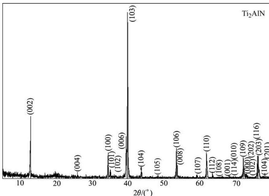
**Fig.2** X-ray diffraction patterns of samples sintered at 1 300 °C analyzed by MDI Jade 5.0 software
