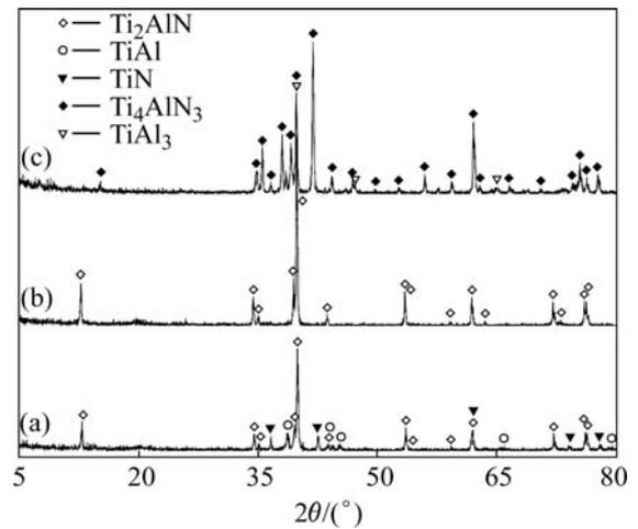
**Fig.1** XRD patters of samples sintered at 1 200 °C (a), 1 300 °C (b) and 1 400 °C (c)
