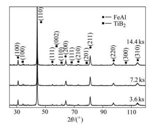
**Fig.3** XRD patterns of 50 h milled Alloy 2 annealed at 1 373 K for different time
