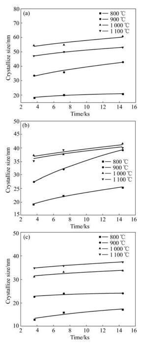
**Fig.4** Grain growth curves in isothermal annealing of MAed Alloy 1 (a), Alloy 2 (b) and Alloy 3 (c) annealed at 1 073–1 373 K for 1–4 h
