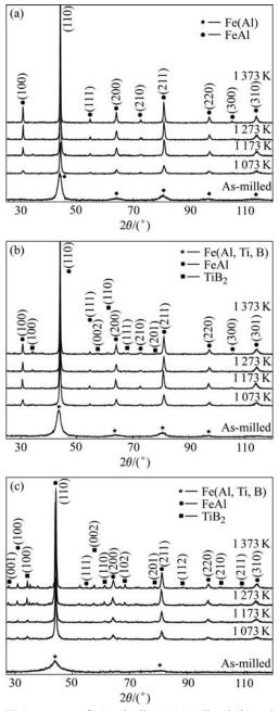
**Fig.2** XRD patterns of MAed Alloy 1 (a), Alloy 2 (b) and Alloy 3 (c) annealed at 1 073, 1 173, 1 273 and 1 373 K for 4 h
