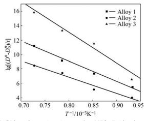
**Fig.5** Plots of  $lg[(D^n - D_0^n)/t]$  against 1/T for FeAl grains
