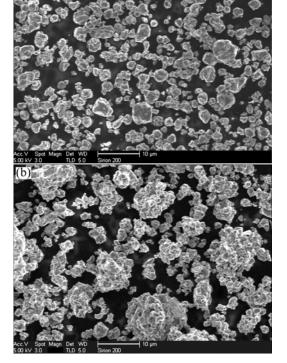
**Fig.1** SEM images of 50 h milled Alloy 2 powders before (a) and after (b) heat treatment at 1 173 K for 4 h
