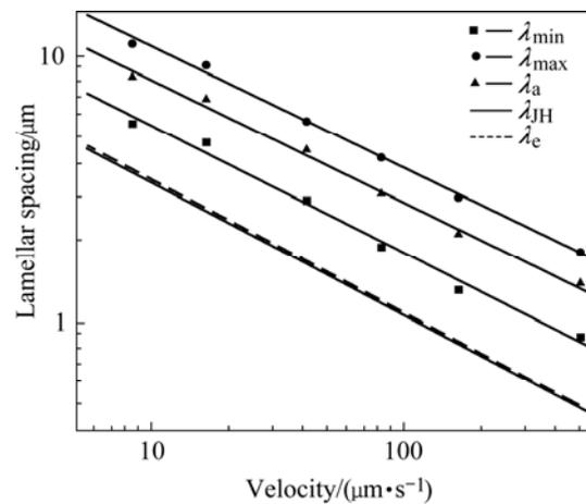
**Fig.1** Comparison of calculated and measured[11] lamellar spacings for Al-Si eutectic at different growth rates
