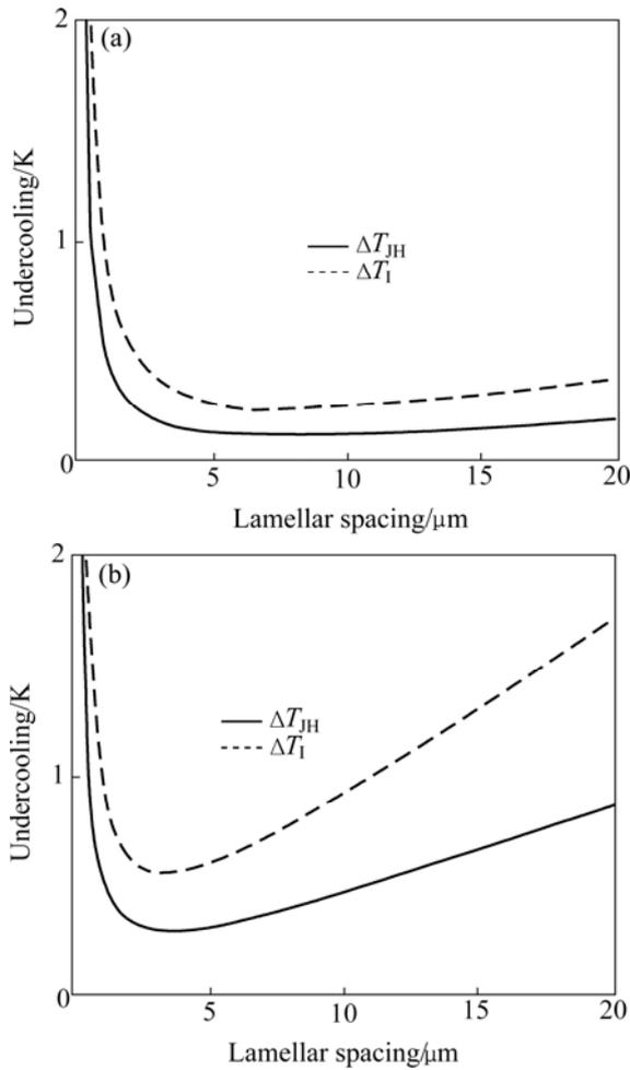
**Fig.2**  $\Delta T_I$  and  $\Delta T_{JH}$  vs lamellar spacing for Al-Si eutectic alloy at  $v=2.0 \mu\text{m/s}$  (a) and  $10.0 \mu\text{m/s}$  (b)
