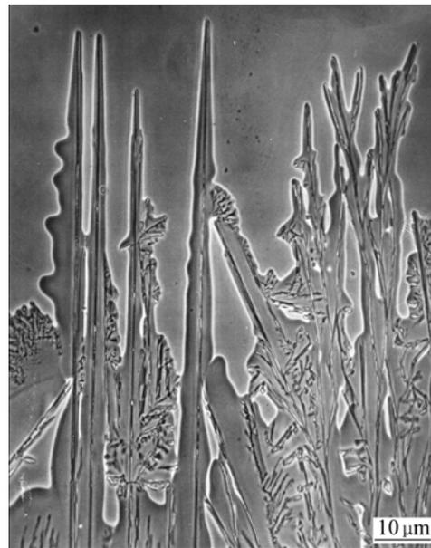
**Fig.4** Interface morphology during directional solidification of SCN-bermol alloy, which resembles aluminum-silicon system [22]
