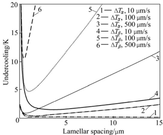
**Fig.3** Average undercooling vs lamellar spacing for eutectic phases in Al-Si eutectic alloy at different velocities
