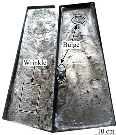
**Fig. 3** Typical surface defects of composites cast in air
