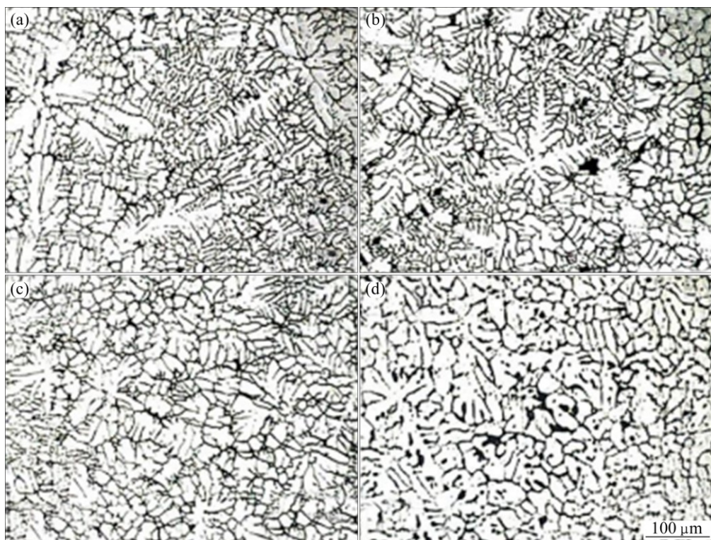
Fig. 4 Microstructures of refined specimens with 0.01% B (a), 0.05% B (b), 0.1% B (c) and 0.3% B (d)
