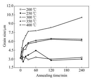
**Fig.5** Grain size versus annealing time at different annealing temperatures of AZ31 after ARB at 300  $\,^{\circ}\text{C}$
