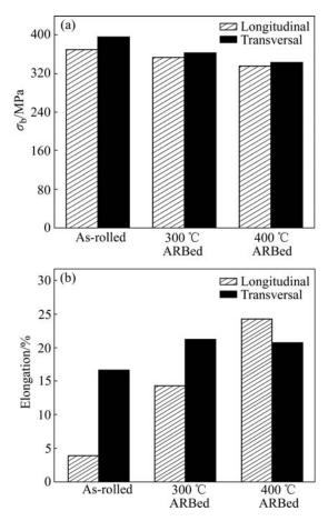
**Fig.3** Mechanical properties of AZ31 after being ARBed at  $300^{\circ}$ C and  $400^{\circ}$ C: (a) UTS; (b) Elongation
