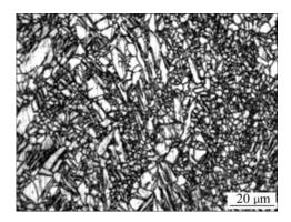
Fig.1 Optical microstructure of as-rolled AZ31
