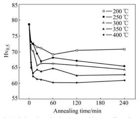
Fig.7 Variation in microhardness with annealing time at different temperatures of AZ31 after being ARBed at 300  $\,^\circ\!C$
