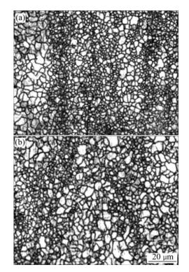
**Fig.2** Typical microstructures of AZ31 after ARB for three cycles at different temperatures: (a) 300 °C; (b) 400 °C
