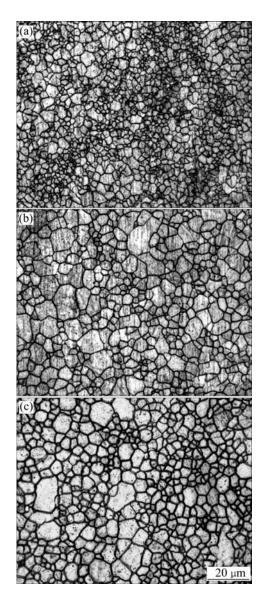
**Fig.6** Microstructures of ARBed AZ31 sheets after annealing under different conditions: (a) 250 °C, 240 min; (b) 300 °C, 10 min; (c) 400 °C, 5 min
