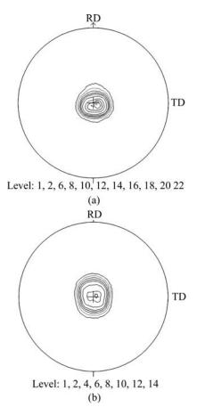
**Fig.4** (0002) pole figures corresponding to AZ31 Mg alloy sheets: (a) As-rolled; (b) Three-cycle ARBed at 300  $\degree$ C
