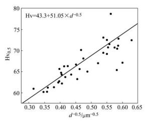
**Fig.8** Values of  $Hv_{0.5}$  versus reciprocal of square root of grain size for all annealing conditions
