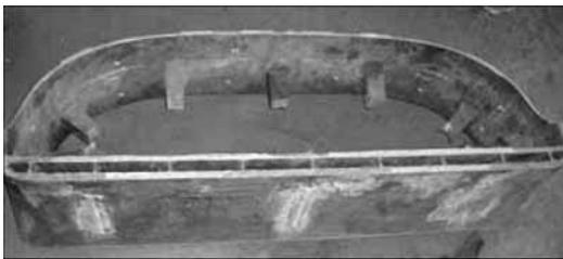
**Fig.7** Typical large thin-walled A357 casting produced by control system
