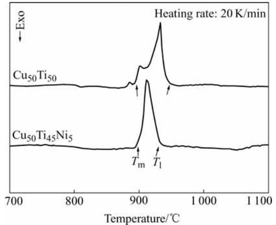
Fig.4 DSC traces of melt-spun  $\text{Cu}_{50}\text{Ti}_{50}$  and  $\text{Cu}_{50}\text{Ti}_{45}\text{Ni}_5$  amorphous alloys
