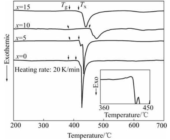
Fig.3 DSC traces of  $\text{Cu}_{50}\text{Ti}_{50-x}\text{Ni}_x$  ( $x=0, 5, 10, 15$ ) amorphous alloys and amplified DSC trace of  $\text{Cu}_{50}\text{Ti}_{45}\text{Ni}_5$  ribbon (inset)
