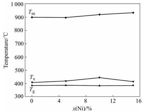
Fig.5 Thermal analysis of melt-spun  $\text{Cu}_{50}\text{Ti}_{50-x}\text{Ni}_x$  ( $x=0, 5, 10, 15$ ) alloys
