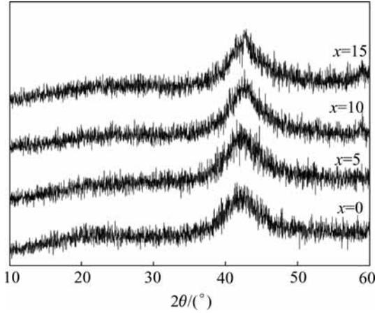
Fig.1 XRD patterns of melt-spun  $\text{Cu}_{50}\text{Ti}_{50-x}\text{Ni}_x$  ribbons
