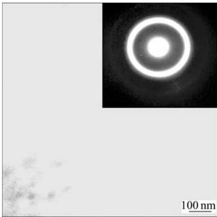
Fig.2 Bright field TEM image and selected area diffraction pattern of  $\text{Cu}_{50}\text{Ti}_{50}$  ribbon
